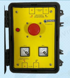
Once the cables from the welding power-source are connected, turn on the machine and check to see that the volt meter registers (no need to connect the welding cables to the diver yet). The volt meter is a zero centred meter and so the needle should rise in an upwards direction. If the meter falls (drops) in a downward direction, then the cables are not matched like-for-like! (Check connections and/or polarity switch and re-test).
